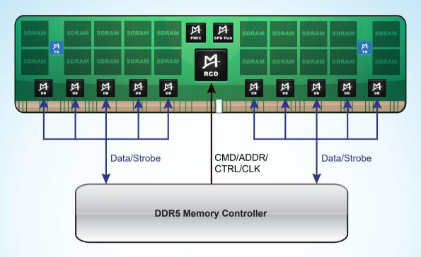
Notes: Here shows the application of TS on the DDR5 LRDIMM as an example.
