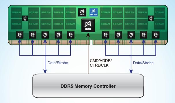
Notes: Here shows the application of SPD Hub on the DDR5 LRDIMM as an example.
